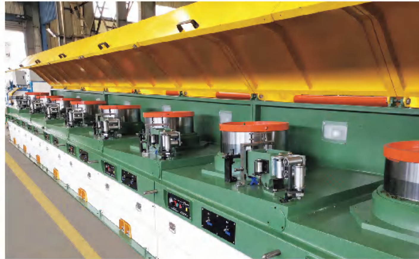
LZ560-900连续直进式拉丝机 Continuous Straight Wire Drawing Machine
