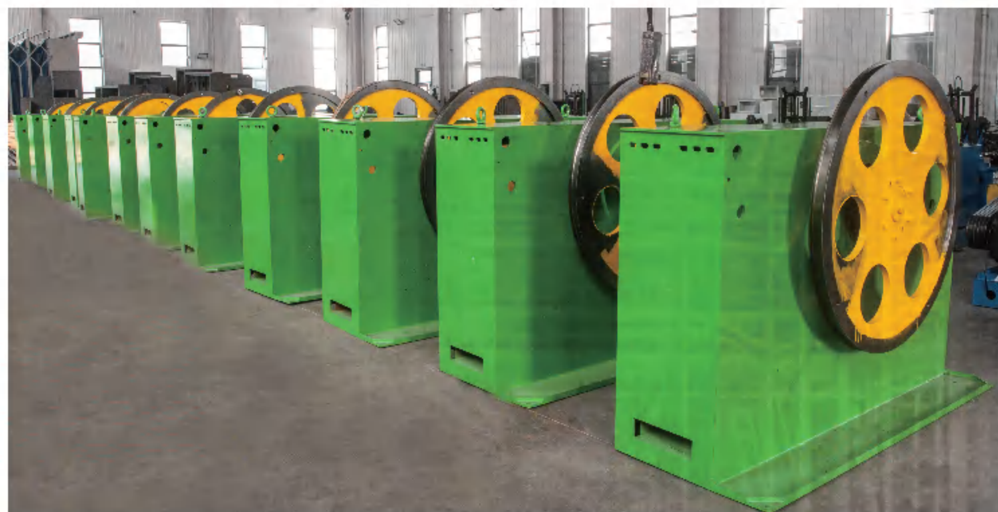
12头收线机（高碳钢弹簧线） 12-head take-up machine (for drawing high-carbon steel spring wires)
