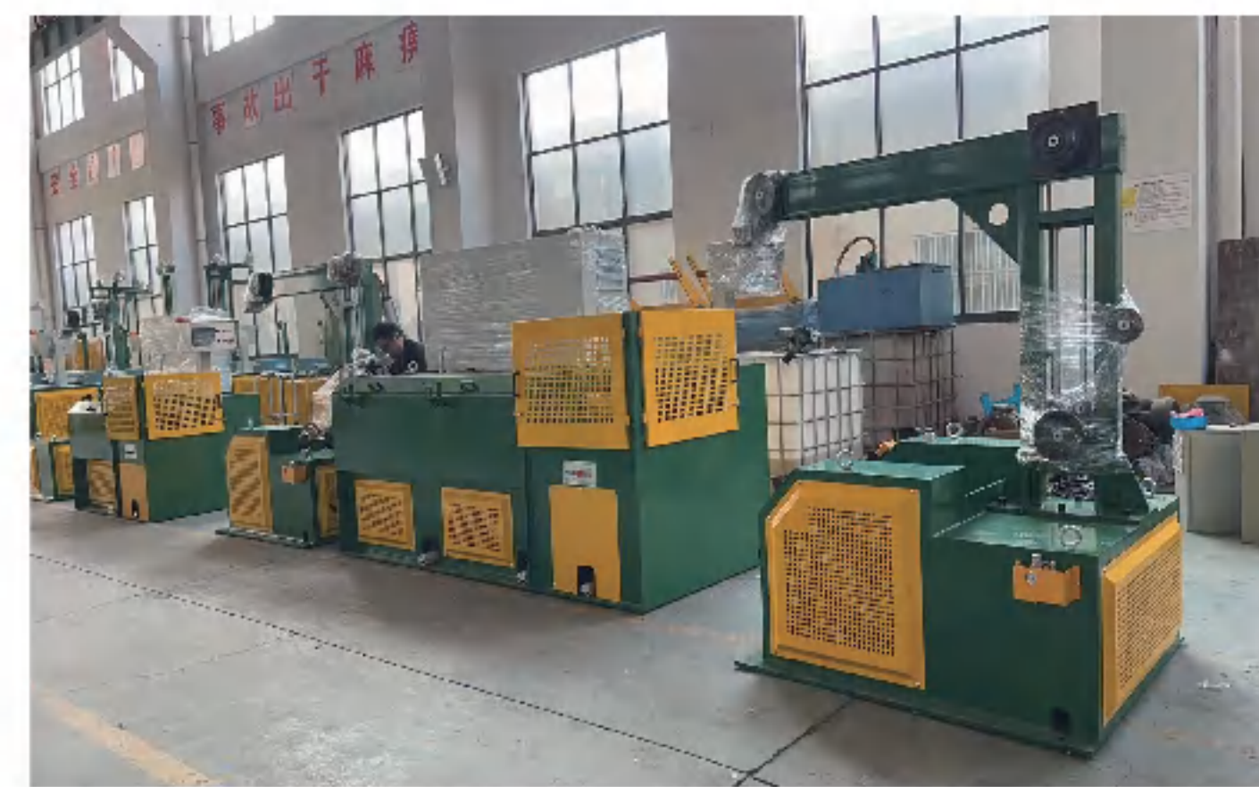
合金铜线专用水箱拉丝机 Water tank wire drawing machine specially for alloy copper wires
