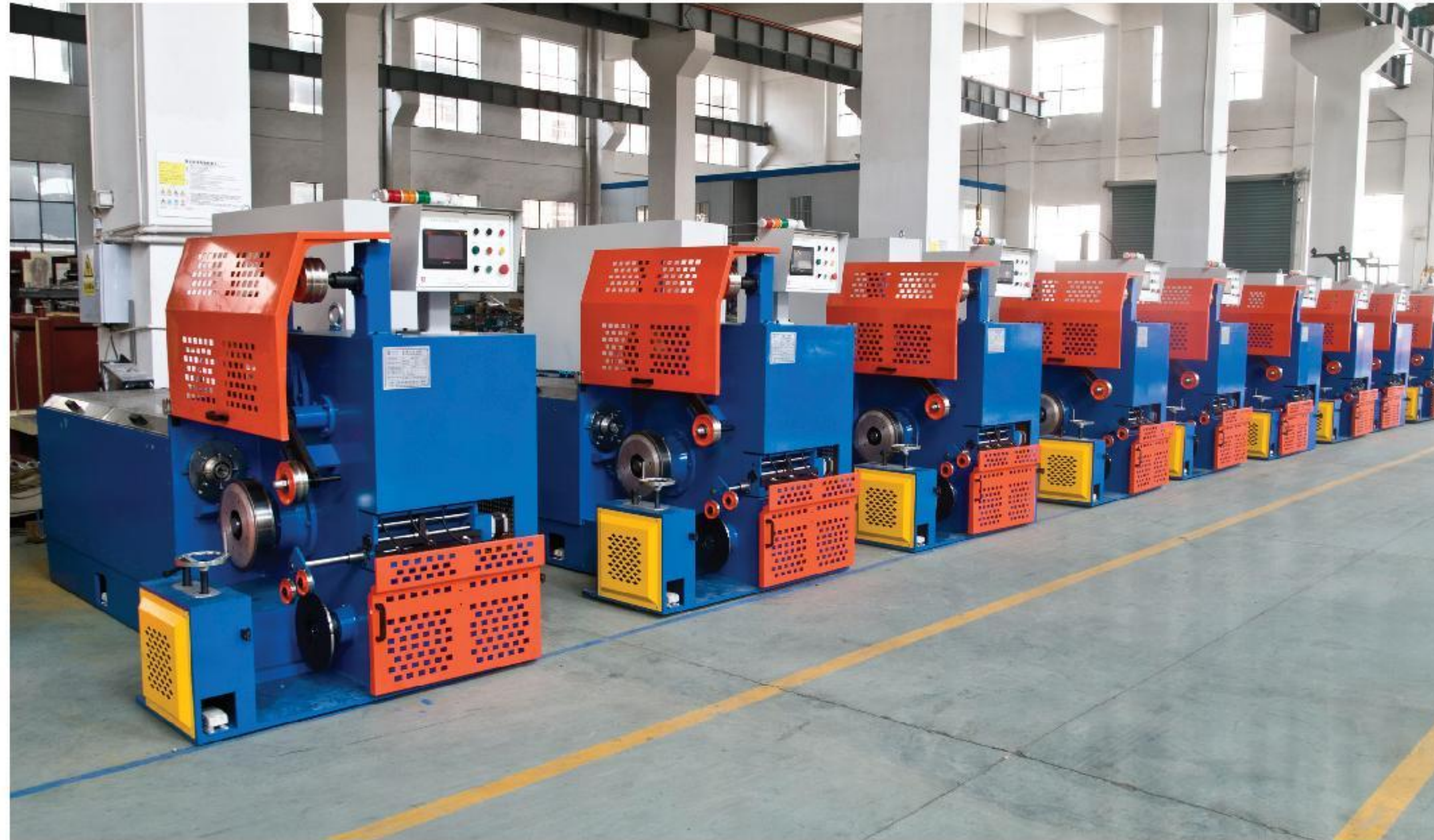
PHOSPHATING HIGH-CARBON STEEL WIRE ROPE-MAKING WIRE DEDICATED WATER TANK DRAWING MACHINE 磷化高碳钢丝及（制绳丝）专用水箱拉丝机
