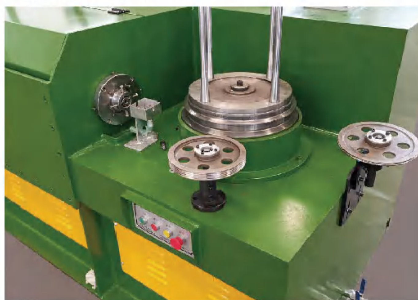
弹簧线拉丝机 Spring Wire Drawing Machine
