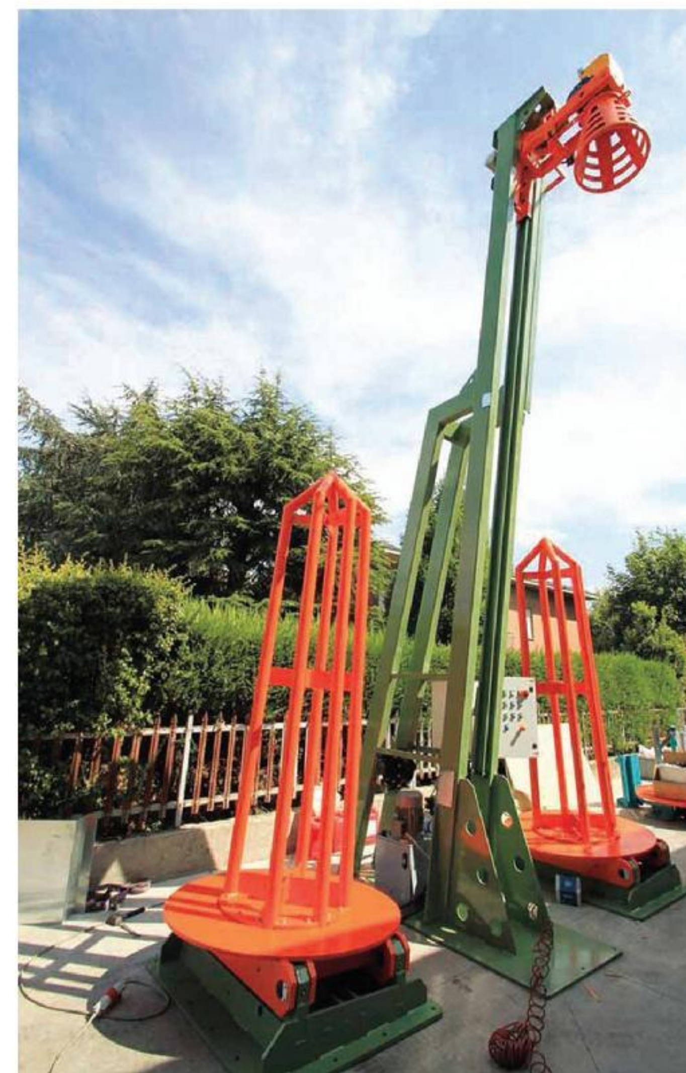
液压双工位大线放线架 Hydraulic double-station large wire decoying rack
