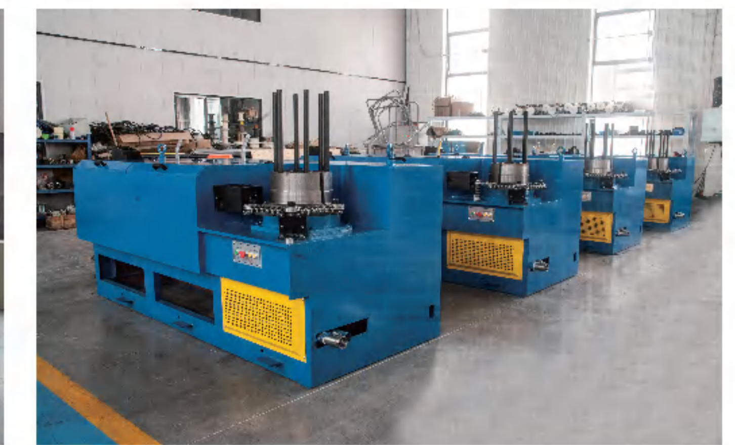
ZT-17D/350水箱拉丝机（拉弹簧线） ZT-17D/350 Water Tank Wire Drawing Machine (for drawing spring wires)
