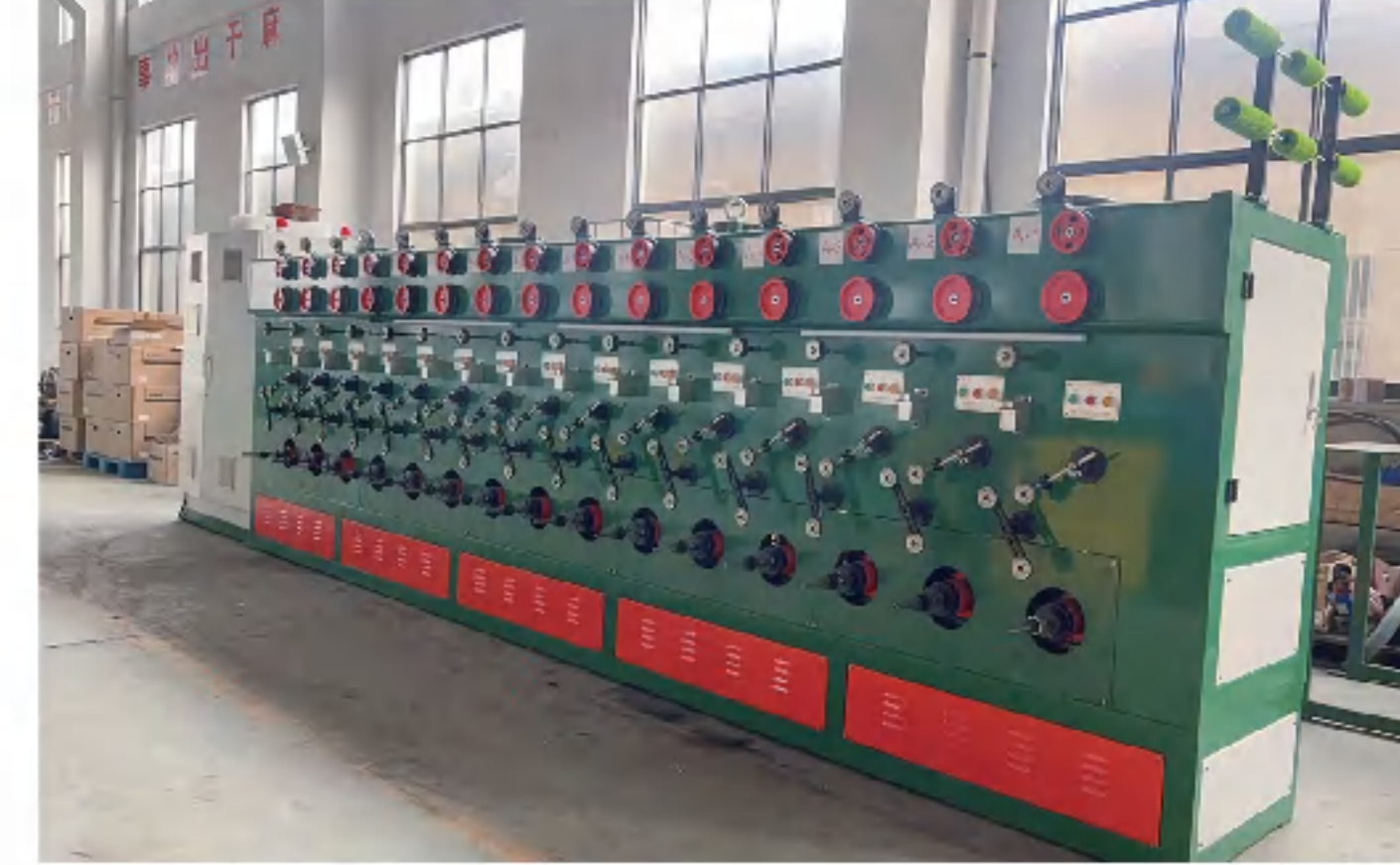
不锈钢丝管式退火炉及收放线设备 Stainless Steel Wire Tubular Annealing Furnace & pay-off And Take-up Equipment
