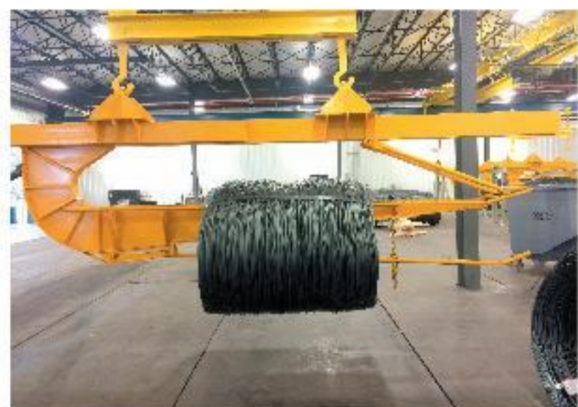
C型放线架 C Type Pay-off Device
