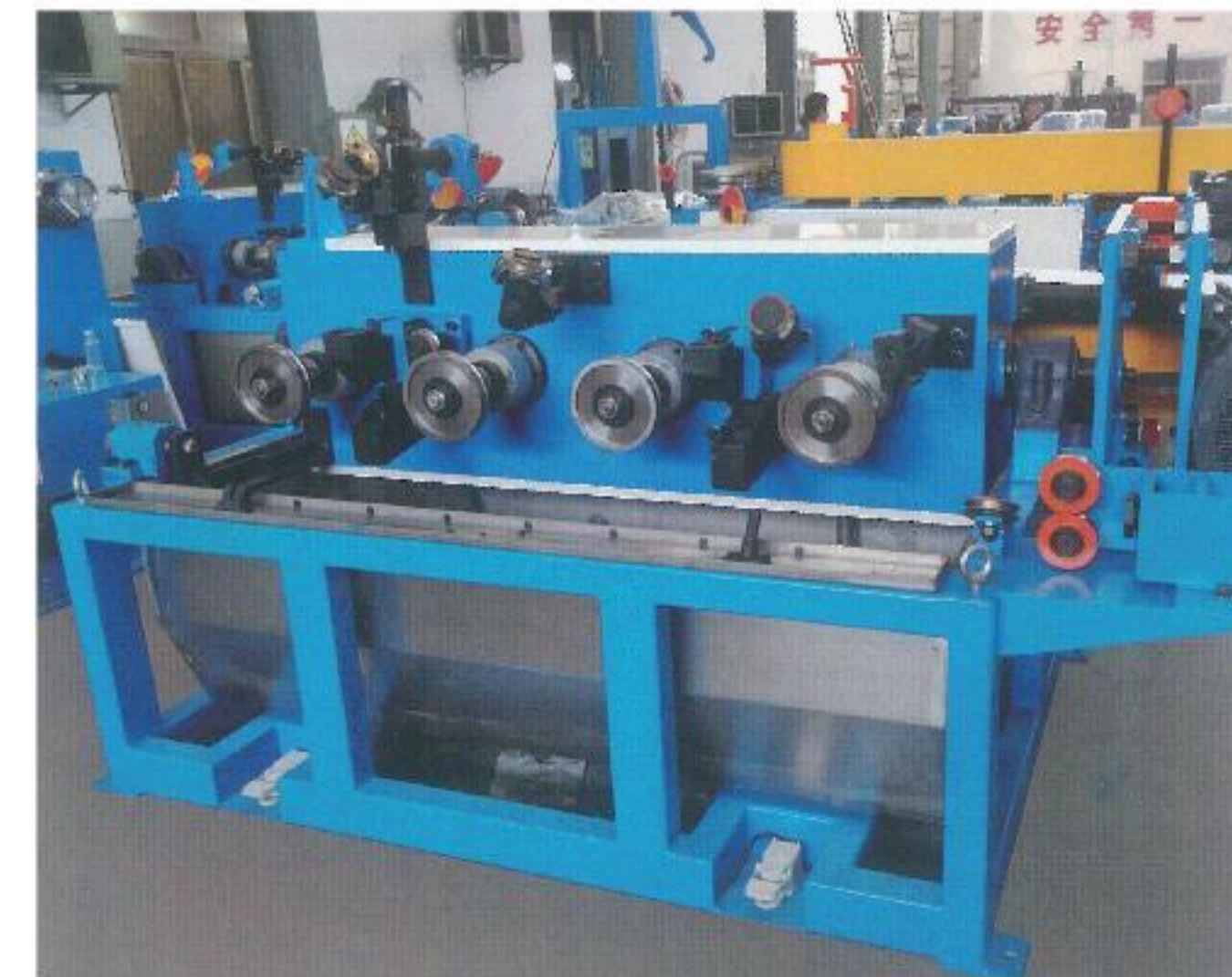
翻转式水箱拉丝机 Turnover Type Wet Wire Drawing Machine
