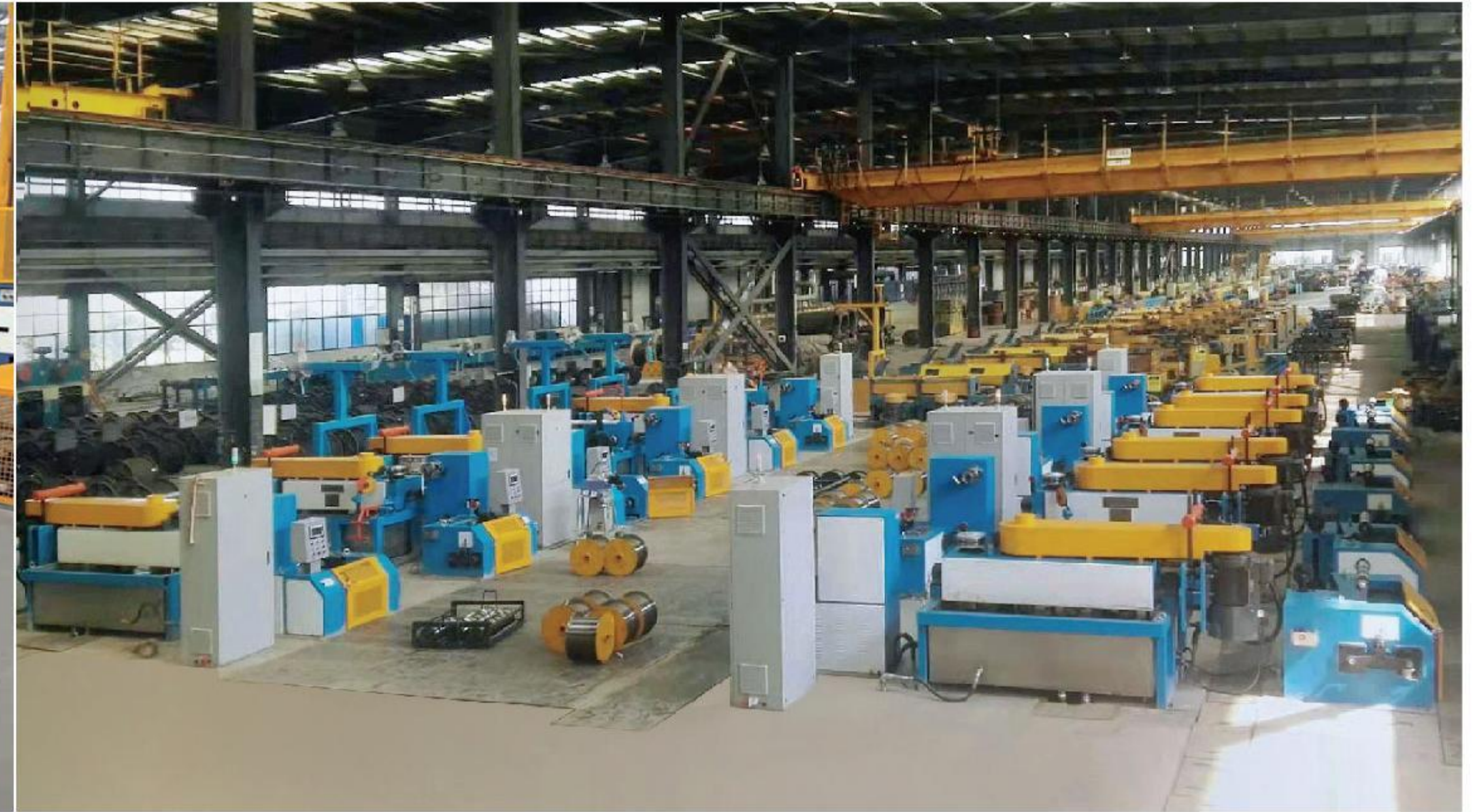
翻转式水箱拉丝机 Turnover Type Wet Wire Drawing Machine
