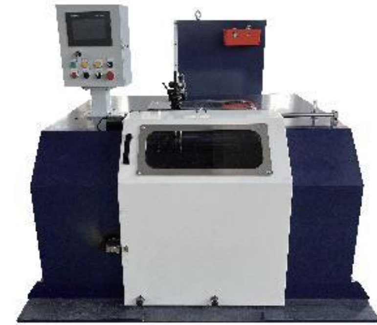
工字轮收线机 Spool take-up machine
