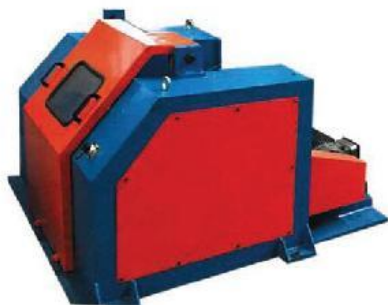
SG630工字轮放线机 SG630 Bobbin Pay-off Machine
