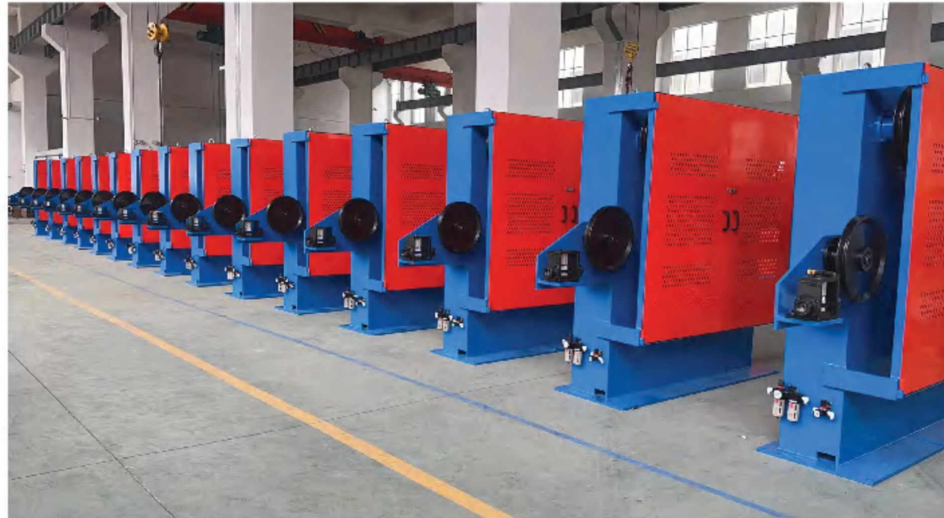
立式放线机 Vertical Unwinding Machine
