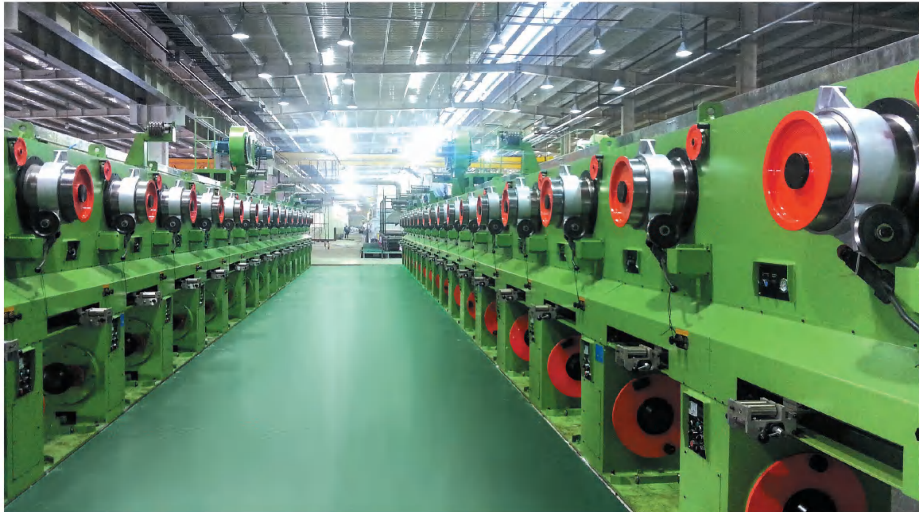
双筒收线机 Double drum take-up machine
