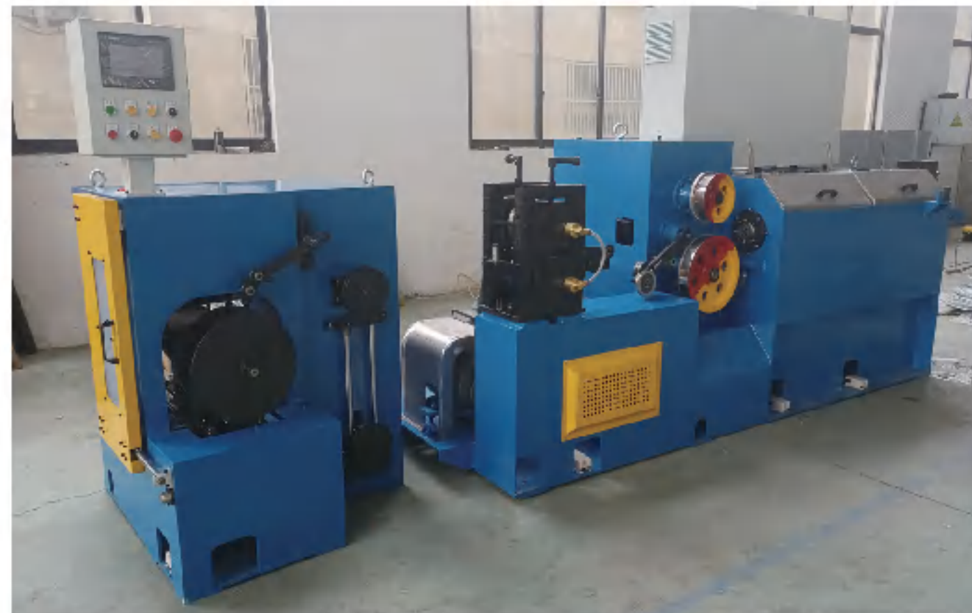
气排钉扁丝拉丝机 Air nail flat wire drawing machine
