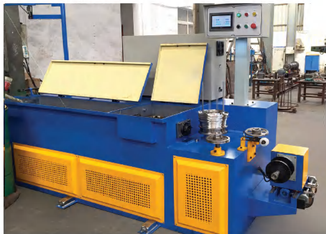
弹簧线拉丝机 Spring Wire Drawing Machine
