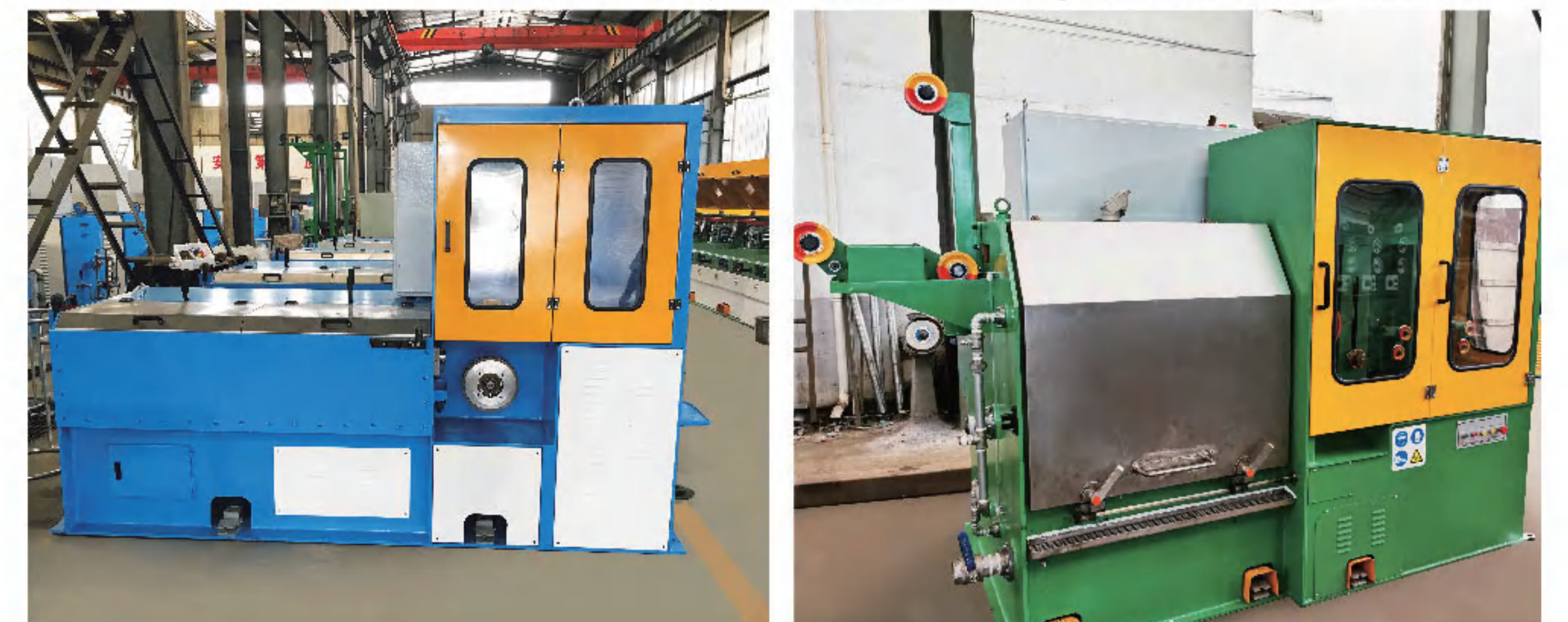
碳钢丝双出线水箱拉丝机 Carbon steel double wire water tank wire drawing machine
