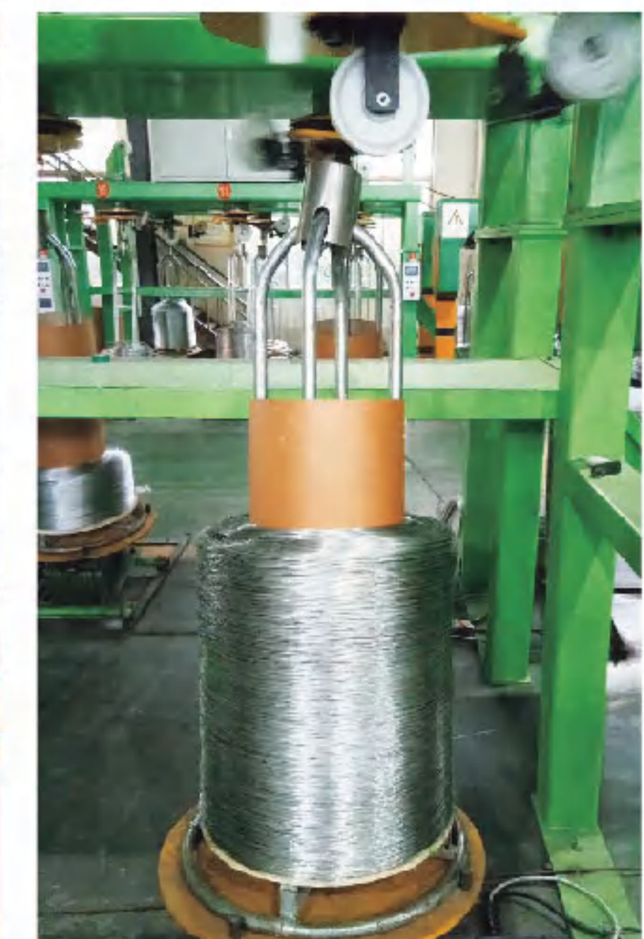
倒立式丝收线机 Inverted take-up machine
