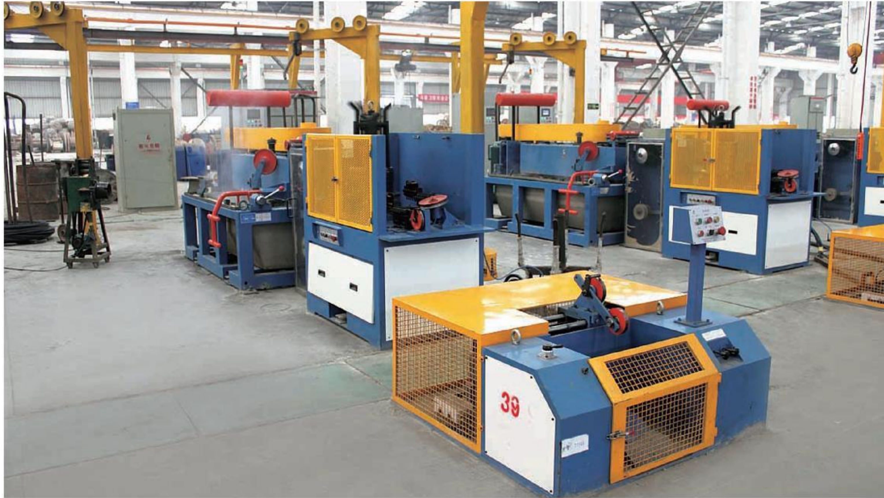
翻转式水箱拉丝机+双收线 Turnover Type Wet Wire Drawing Machine
