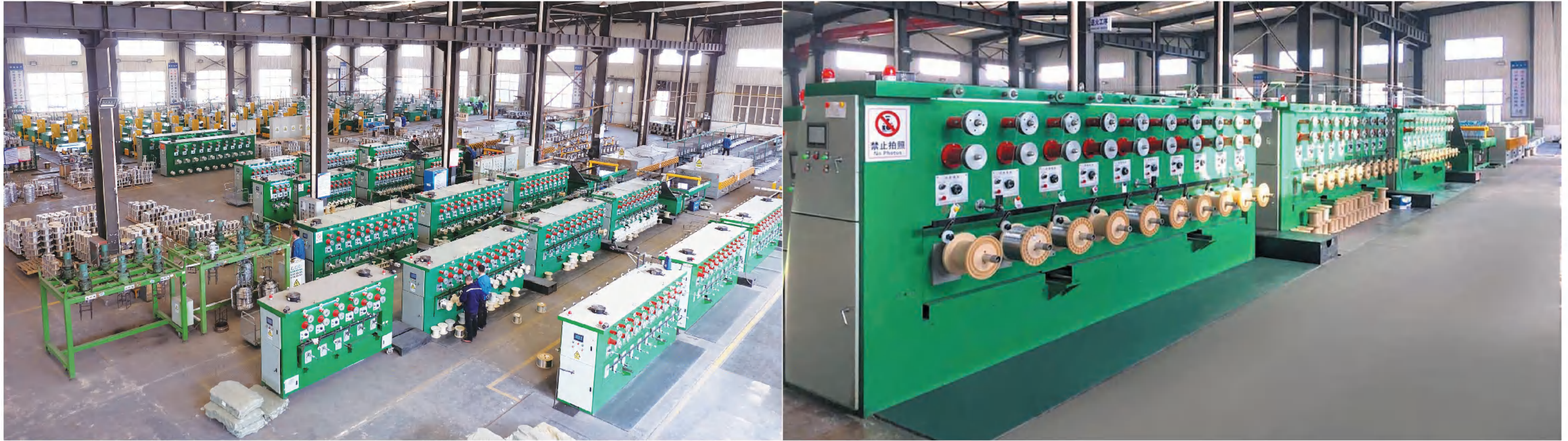
轴动排线收线机 Shaft-driven take-up machine
