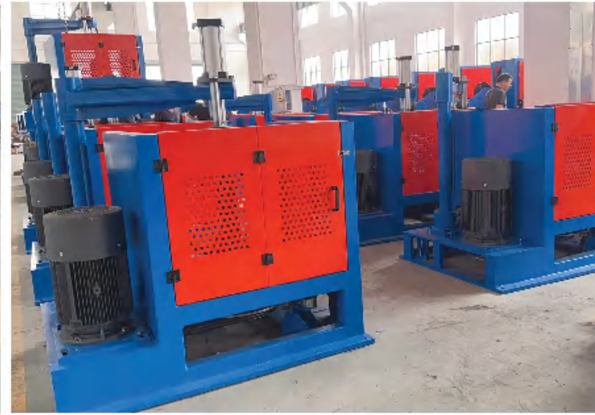
立式放线机 Vertical Unwinding Machine
