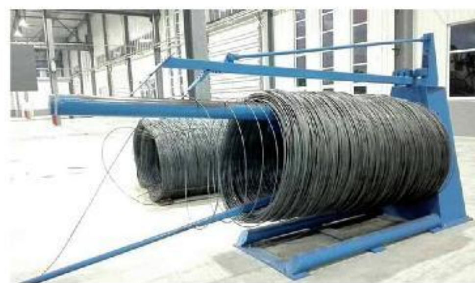
鸭嘴式放线架 Duckbill Type Pay-off Device
