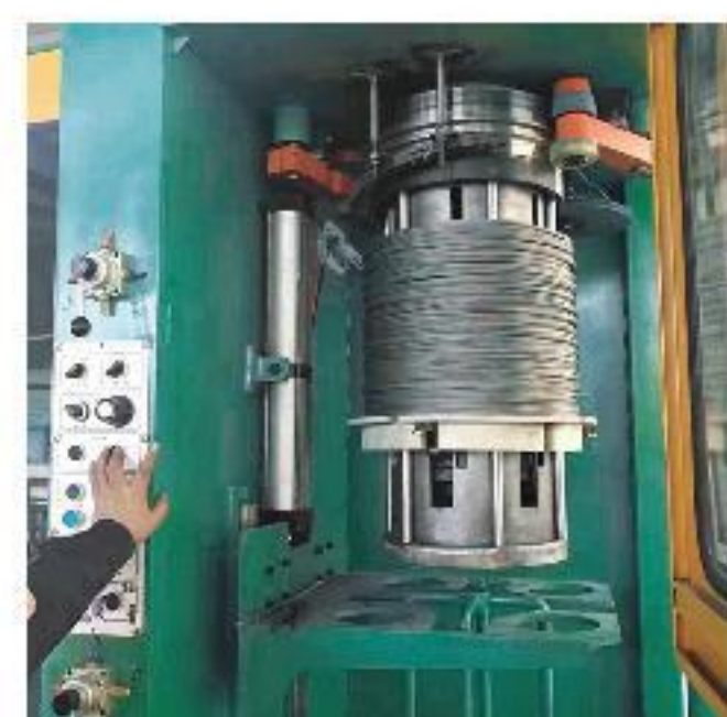
SL400倒立式收线机 SL400 inverted take-up machine
