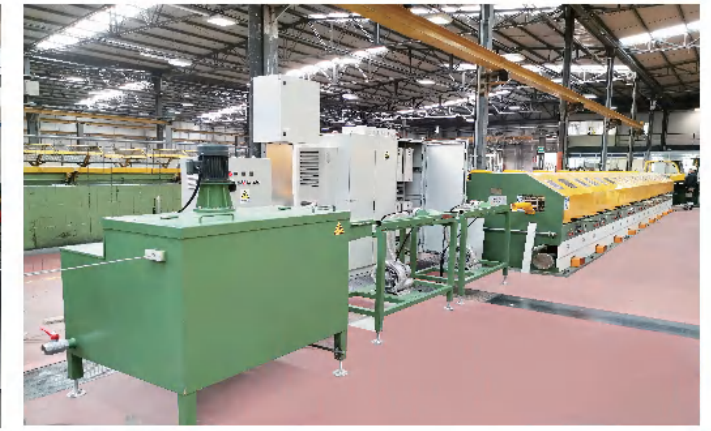
盘条预处理线 Surface Pre-treating Line For Wire Rod
