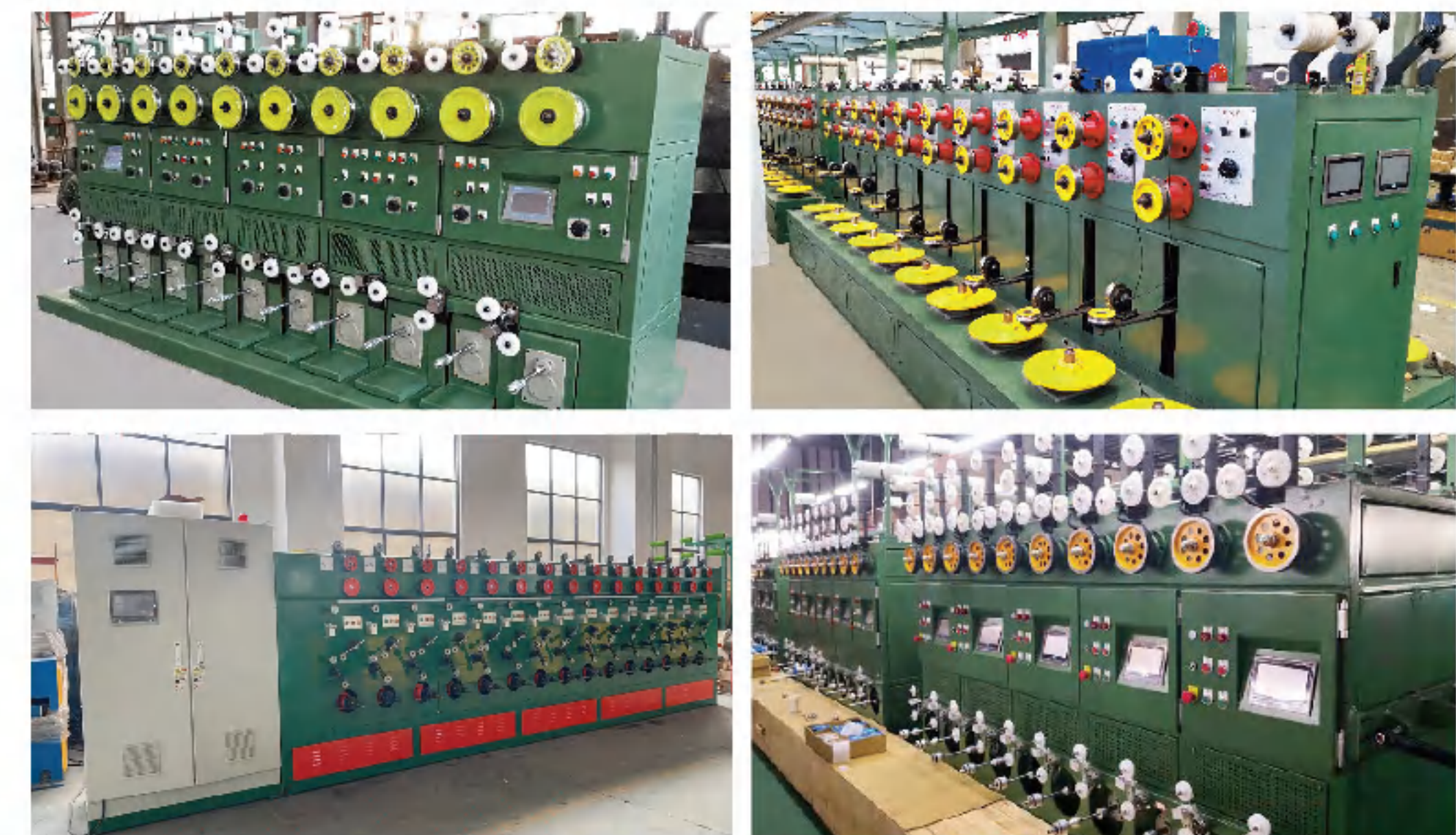
单头单控轴动排线收线机 Single-control shaft driven wire arrangement and winding machine
